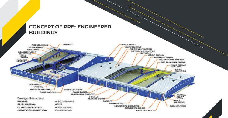
A pre-engineered steel building is a modern technology where the complete designing is done at the factory and the building components are brought to the site in CKD (completely knock down condition) and then fixed/jointed at the site and raised with the help of cranes.
